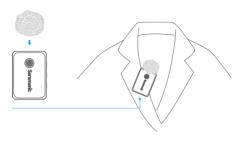
The transmitter comes with a windproof capsule. It can fit an extra fur windshield when you need to enhance wind protection outdoors or in a windy environment.
